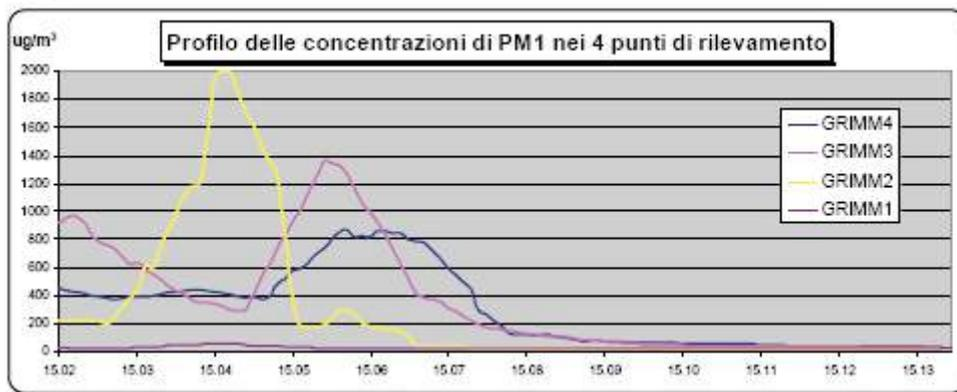
**Grimm 1:** at the air input in the filtering station, **Grimm 2:** 40 m, **Grimm 3:** 80 m, **Grimm 4:** 120 m
